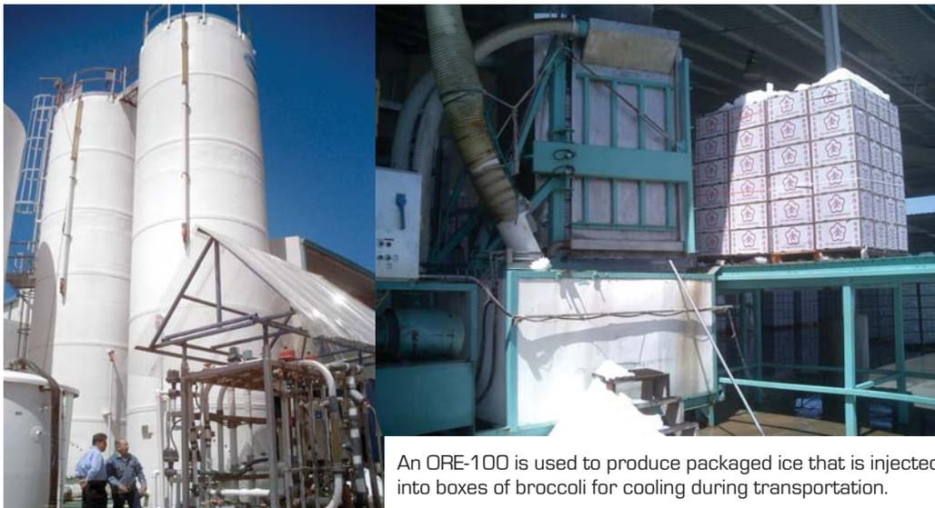
An ORE-100 is used to produce packaged ice that is injected into boxes of broccoli for cooling during transportation.
